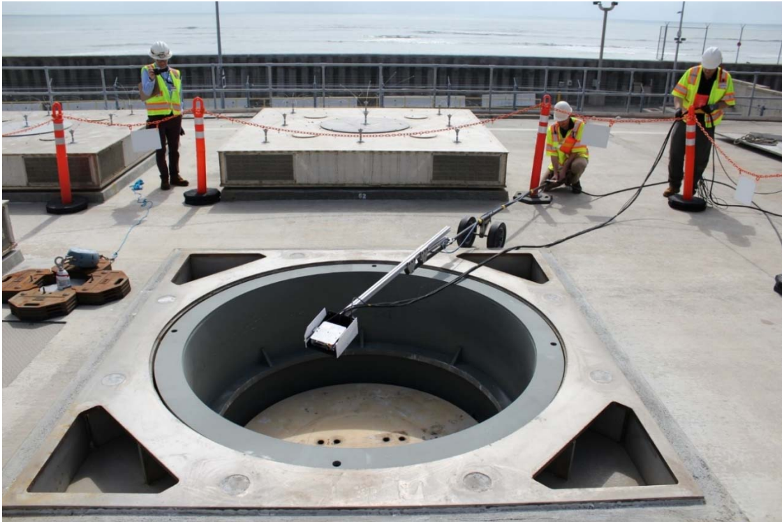
Figure 4 - The inspection robot is held in a delivery tool and placed into the cavity enclosure container to begin the visual inspection of a loaded MPC
