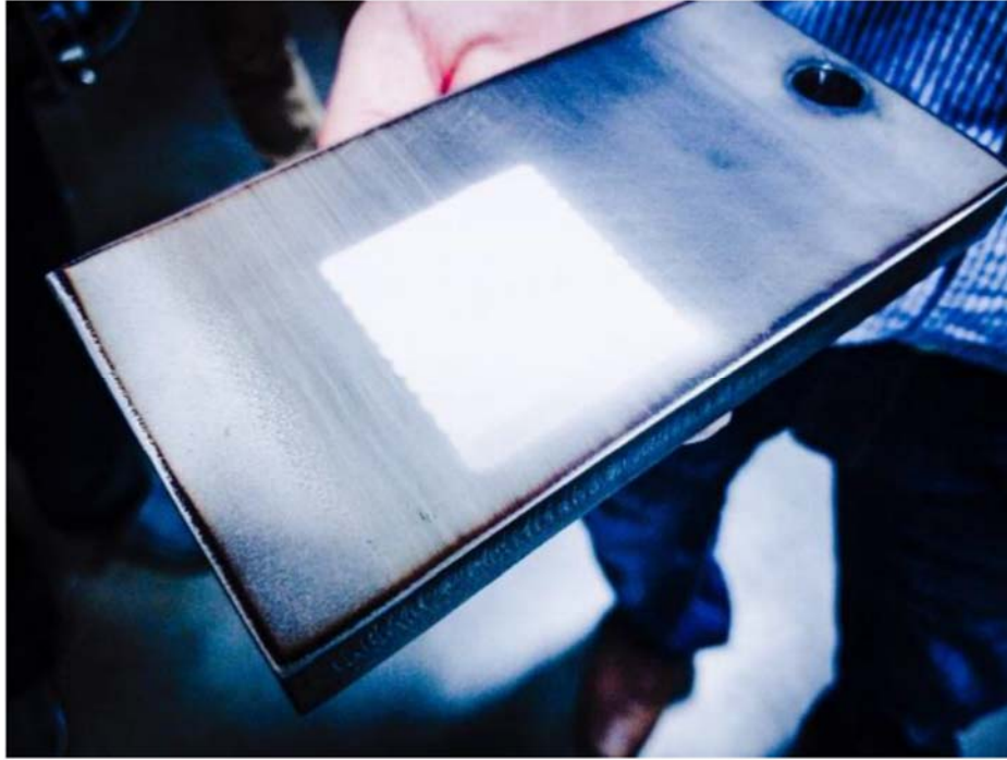
Figure 9 - Canister steel sample with metallic overlay repair
